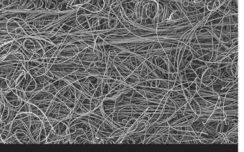
MICROFILAMENTS 4.5 TIMES FINER THAN COMMON POLYESTER FILAMENTS FOR SUPERIOR UNIFORMITY
